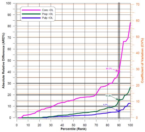
Figure 11.20 – Absolute relative difference vs. percentile (rank) plot for all palladium duplicates (Lustig, 2016)
