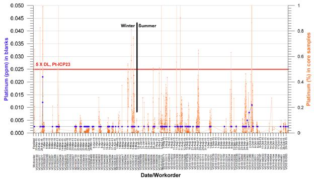
Figure 11.3 – Field blank platinum analyses (blue) and all platinum core analyses (orange) (Lustig 2016).
