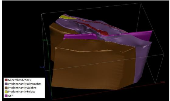
Figure 14.2 presents a 3D view of the lithological and mineralized solids.
