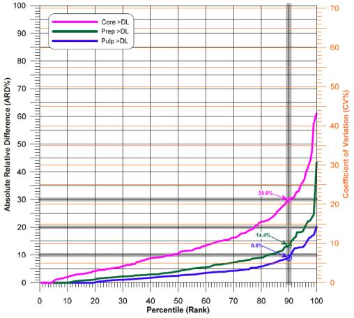
Figure 11.25 – Absolute relative difference vs. percentile (rank) plot for all copper duplicates (Lustig, 2016)
