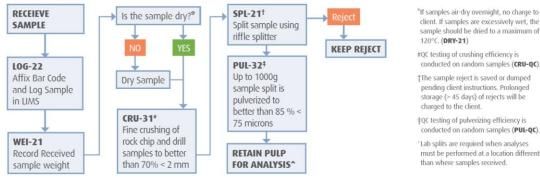
Figure 11.1 – Flow chart of the sample preparation PREP-31B at the ALS Minerals Laboratory
