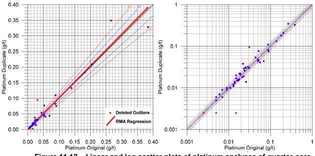
Figure 11.12 – Linear and log scatter plots of platinum analyses of quarter-core field duplicates (Lustig, 2016)
