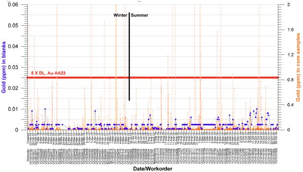
Figure 11.2 – Field blank gold analyses (blue) and all gold core analyses (orange) (Lustig 2016).
