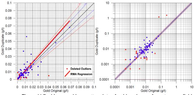
Figure 11.7 – Linear and log scatter plots of gold analyses of quarter-core field duplicates (Lustig, 2016)
