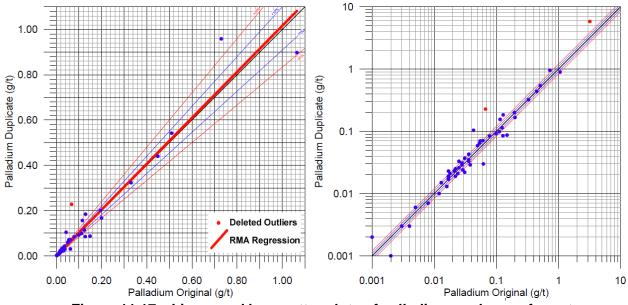
Figure 11.17 – Linear and log scatter plots of palladium analyses of quarter-core field duplicates (Lustig, 2016)
