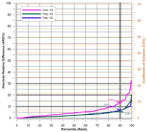
Figure 11.30 – Absolute relative difference vs. percentile (rank) plot for all nickel duplicates (Lustig, 2016)
